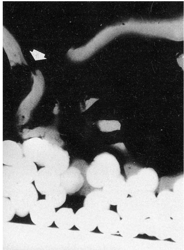
Figure 3 Microradiograph of a hydroxyapatite-coated sample after push-out test (100 \mu\text{m} thickness, X40). The arrow shows a trabecular fracture.
