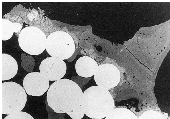
Figure 6 BEI-SEM of a hydroxyapatite-coated sample, X95. Intimate contact between a broad mushroom shape trabeculae and the implant hydroxyapatite-coated surface is shown.
